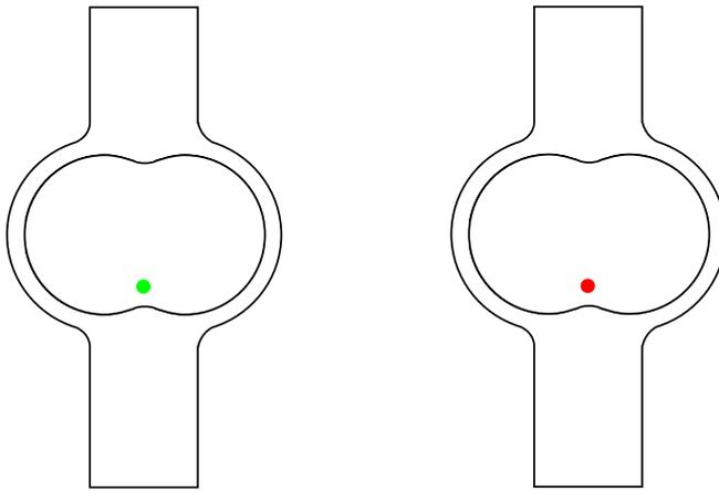
**Green LED** for five seconds, which means that the device has started recording and you can go to sleep or...
