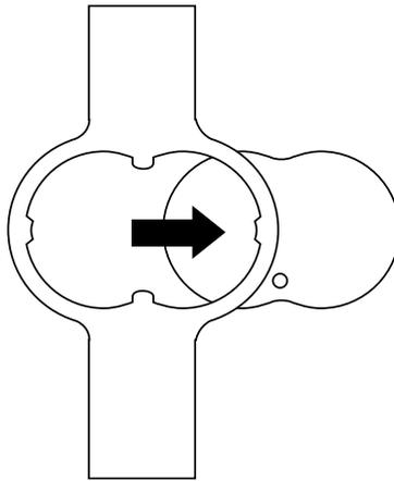
Attach the sensor pod to the bracelet by aligning front of the pod with the wrist side of the band and pressing it into the strap.
